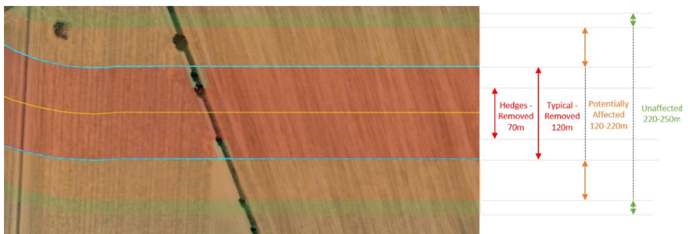
Image 4.13 Vegetation clearance requirements for underground cables
